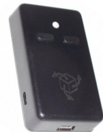
Figure: Commercial IMU (Yost 3-Space). 28 g, 6 cm high.
