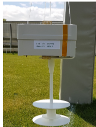
Figure: Infrasound sensor (top box) with noise reduction port (below). \simeq 7 kg, \simeq 40 cm high.
