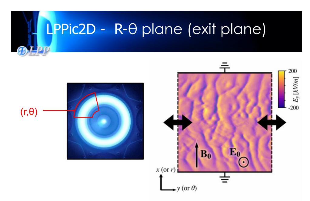
Detailed study of the Electron Cyclotron Drift Instability (ECDI) propagating in the azimuthal direction <sup>13</sup>
