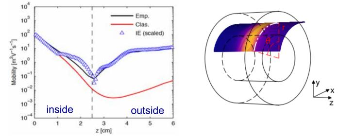
Theoretical works at LPP : new model for the axial mobility of electrons based on kinetic theory
